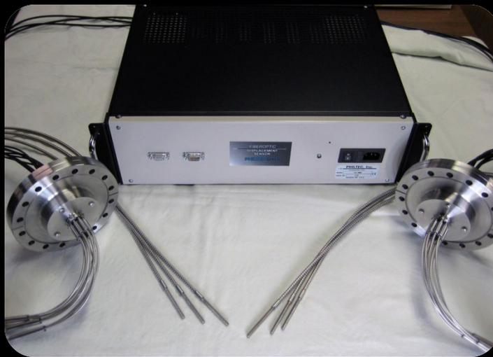
This 6-channel displacement measurement system with vacuum passthru hardware was used to measure displacements and calculate rotations of the satellite's focal plane structure.
