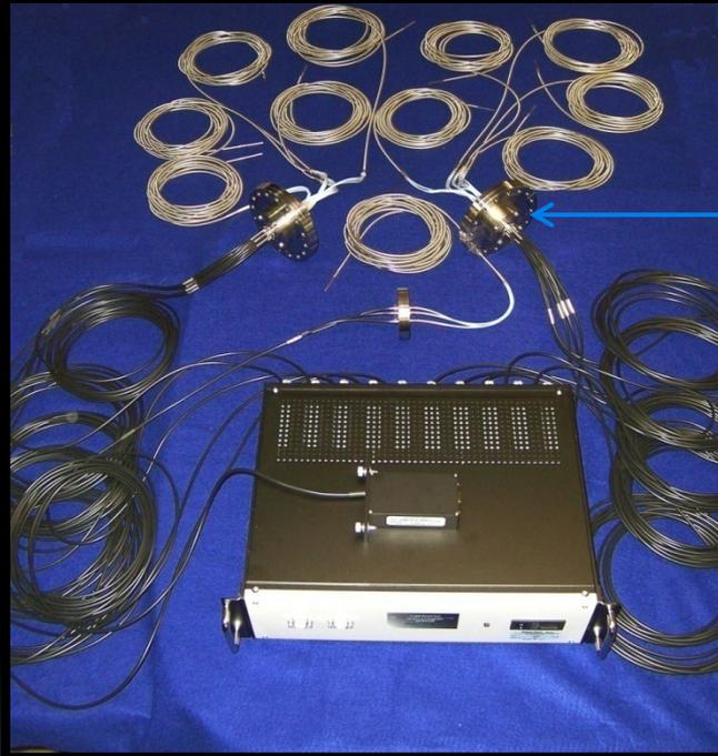
Philtec sensors were used to measure micron level mirror adjustments in high vacuum
