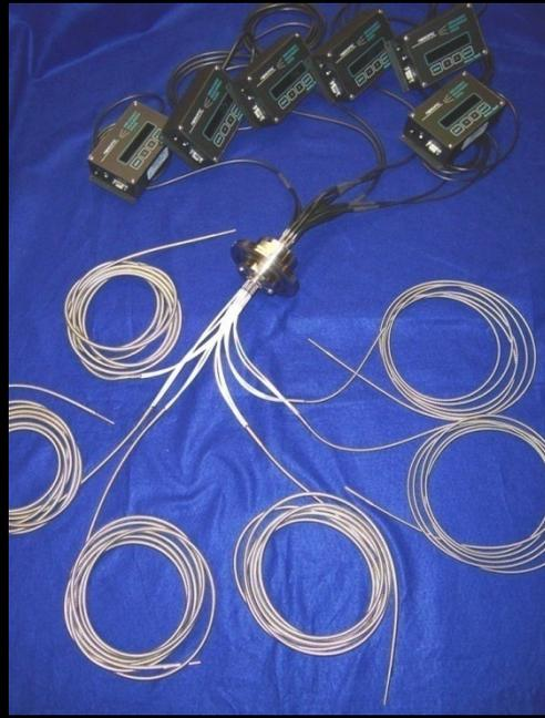
These sensors were used to measure thermal distortions of critical components at low temperatures
