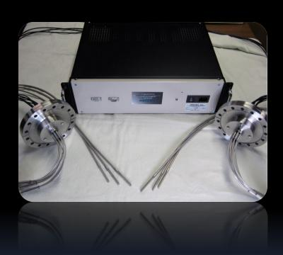
This 6-channel displacement measurement system with vacuum passthru hardware was used to measure displacements and calculate rotations of the satellite's focal plane structure.
