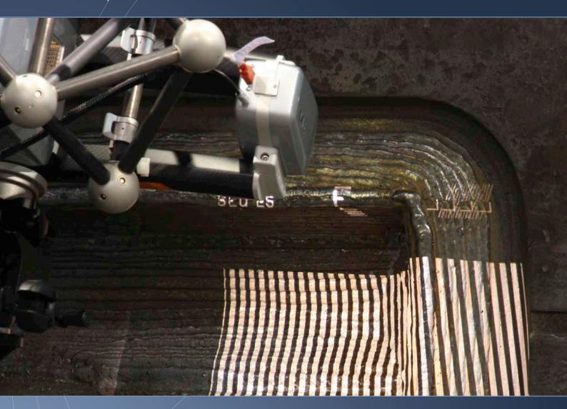
The combination of a **Metronor DUO** portable CMM and a Breuckmann **stereo SCAN**<sup>3D</sup> white-light scanning system offers unknown flexibility and accuracy to users of portable measurement equipment. Probing and scanning has never been so easy and allows sophisticated measuring and inspection tasks on the shop floor.
